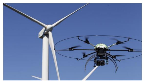
The Aracnocóptero drone detects any incidence on the blades of the wind turbines.
