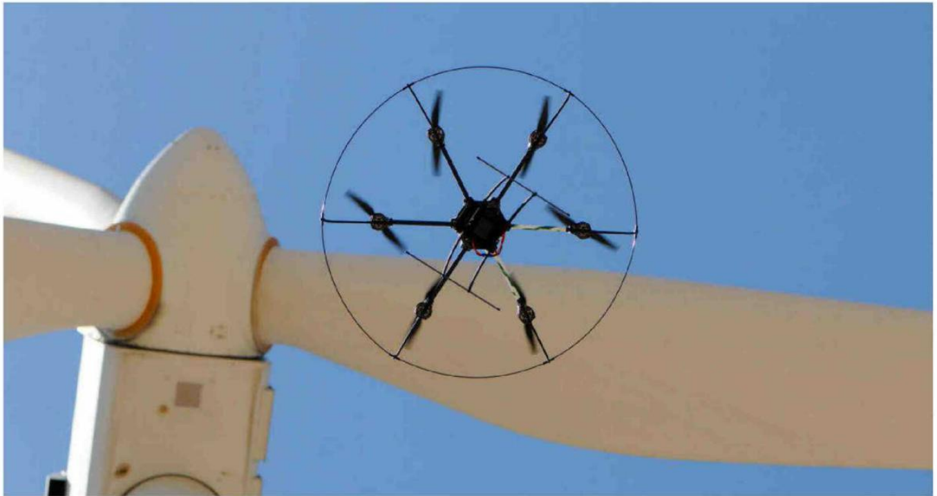
The Aracnocóptero drone, manufactured in the Scientific Park of the University of Salamanca, performs a digital inspection on a wind turbine. ARBÓREA INTELLBIRD
