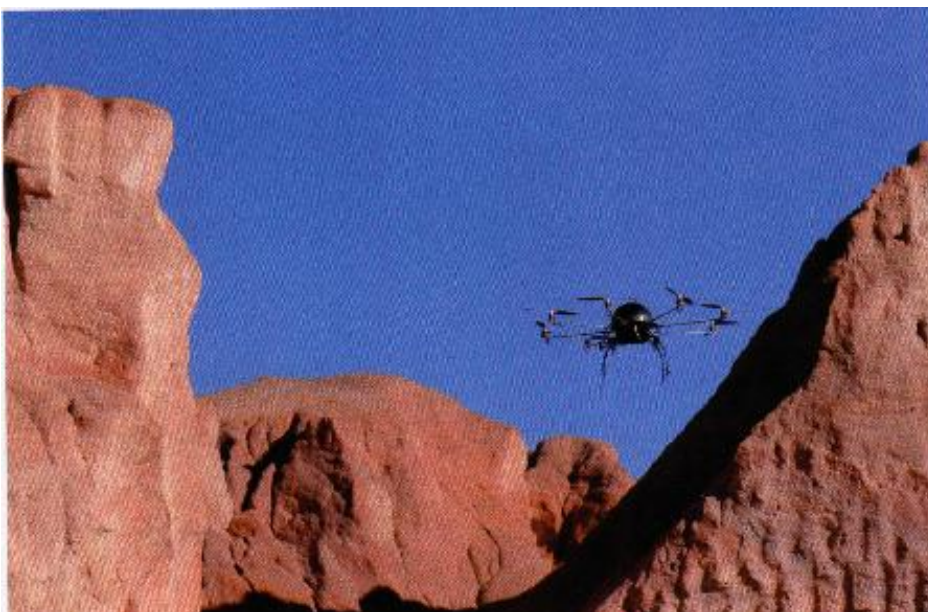
First prototype of Aracnocóptero with foldable chassis made of titanium and carbon fibre.
