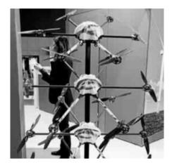
The arachnocopter - marketed by Arbórea, a company in Salamanca owned by Iberdrola - can distinguish defects of up to two millimeters in a windmill.
