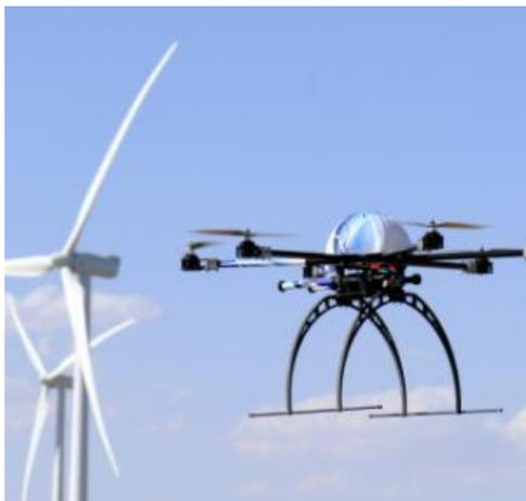
Developed by Arborea Intellbird, a spin-off of the University of Salamanca which also includes Iberdrola, **the drone is equipped with high-resolution cameras and sensors** to control turbines in flight without the need for a pilot, thus reducing scan times and supervision costs.
