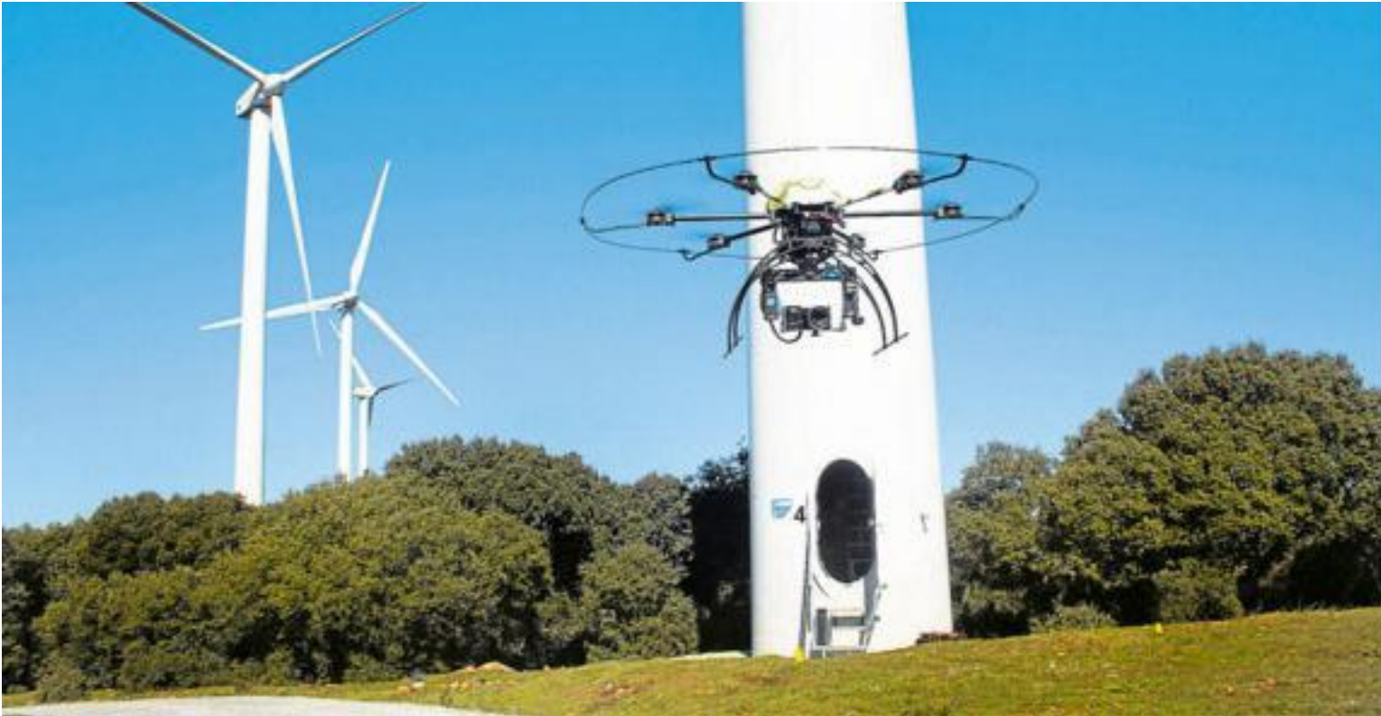
The innovative robot has been designed and executed by a Salamanca company and will save costs in the review of wind turbines. | FOTOS: EÑE
