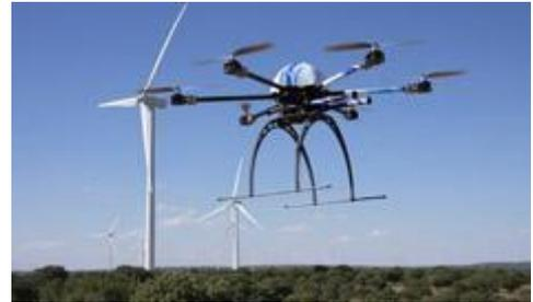
The Eol 6 aircraft model is specifically designed for wind turbine reviews. Photo: Arbórea
